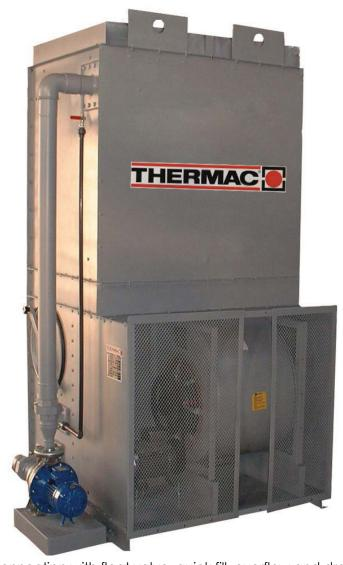
The tank in complete with water make-up connection with float valve, quick fill, overflow and drain. The moisture eliminator are in painted press-bent galvanized sheet metal or in self-extinguishing PVC and eliminate any passage of water droplets.
